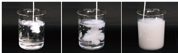
Figure 2. A homogeneous solution of Chiguard® 5582WB in water was achieved simply by gentle stirring
